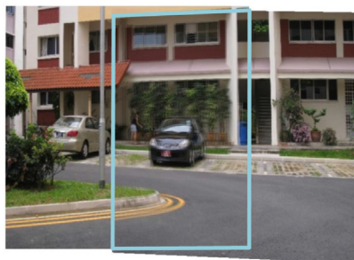
(c) Misalignments in overlapping areas caused by parallax.
