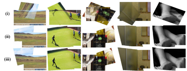
Fig. 9. Failure cases of traditional feature-based methods. (i)(ii): The stitched results of the Global Homography and ours. (iii): The ground truth.
