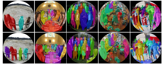
Fig. 7. The detection and segmentation results of the original omnidirectional images (top) and corrected images using our proposed method (bottom) (best viewed in color).
